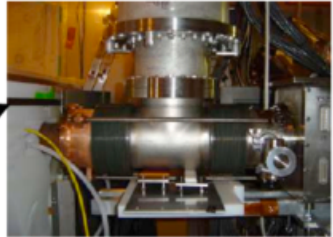
Cryocooler (77K and 4K) Removes heat load from signal cables.
