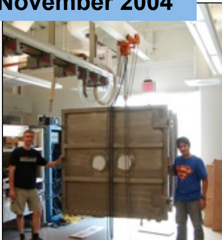
1.5m 3 cubed stainless steel vacuum vessel (UK/USA)
