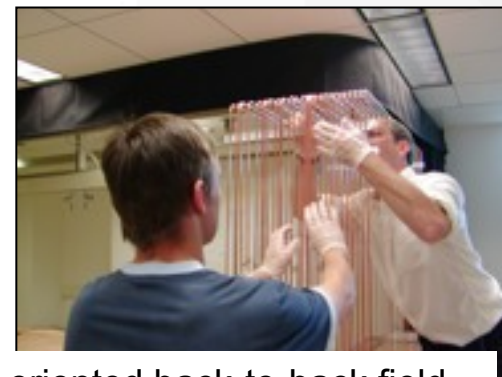
Side-oriented back-to-back field cages with rigid Cu piping.
