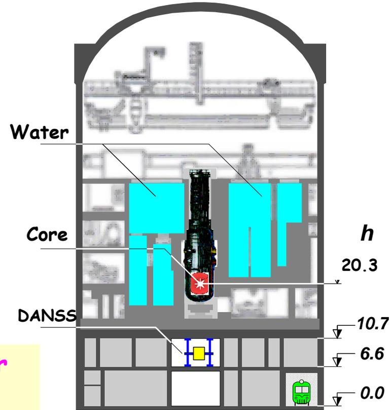
DANSS is installed on a movable platform under 3.1 GW WWER-1000 reactor
