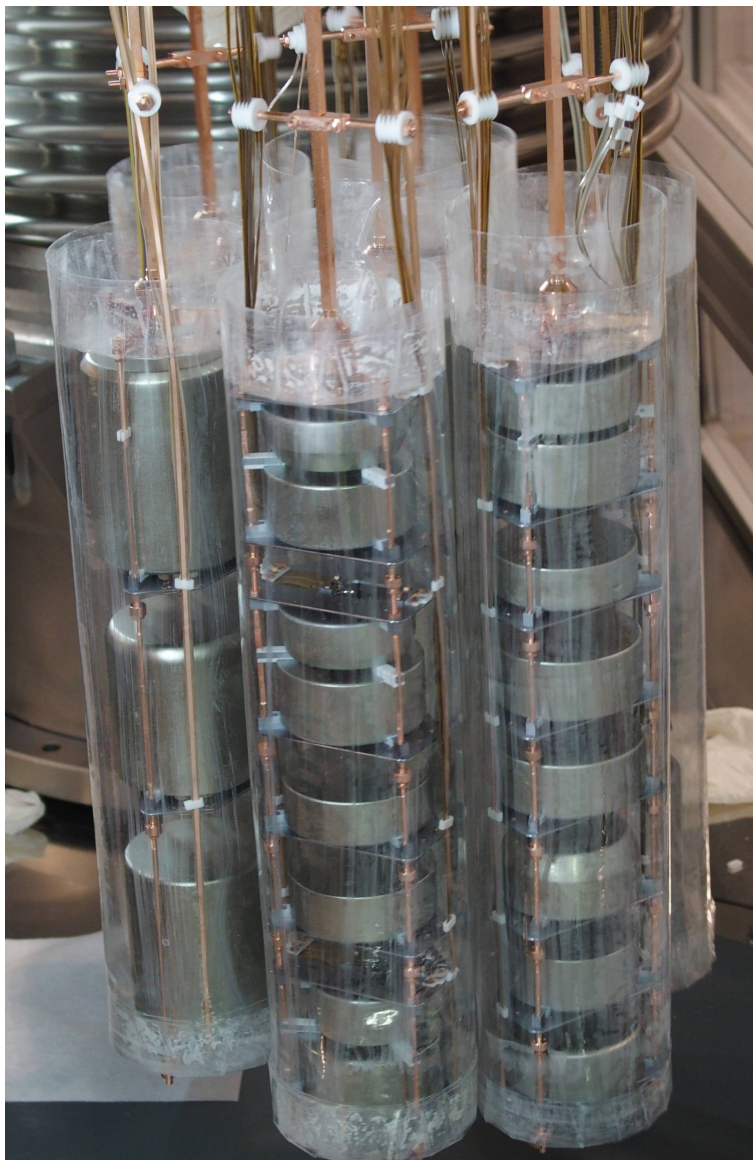
Extended Data Fig. 3. — GERmanium Detector Array GERDA — Photo of the assembled detector array with a string of coaxial detectors (left) and BEGe detectors (middle and right). Each string is enclosed by a cylindrical nylon shroud covered with a wavelength shifter.
