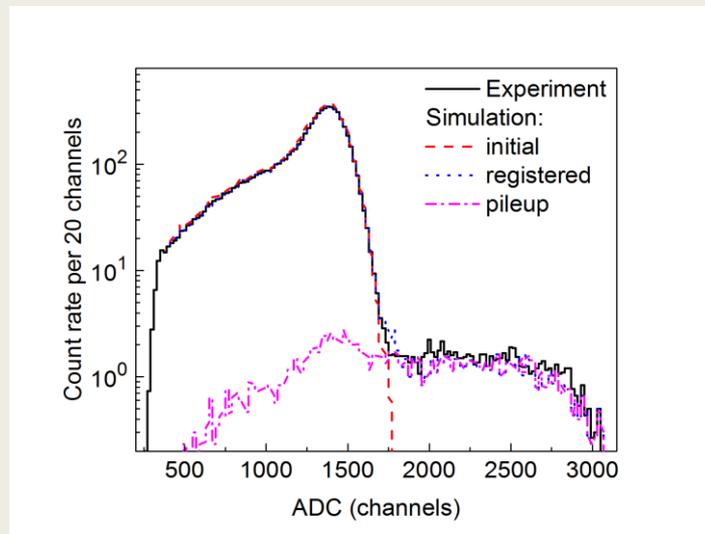
Monte-Carlo simulation using real spectrum and pulser calibration
