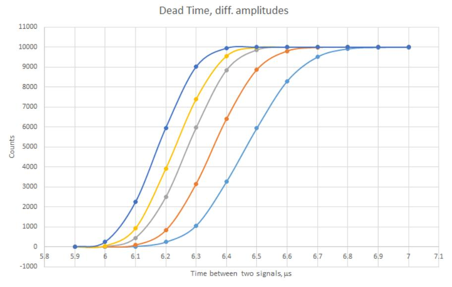
Dead time calibration by pulser and two delayed signals
