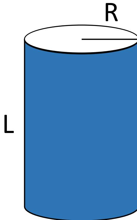
For typical ADMX-HF cavity, L/R=5, enhancement factor = 6.
