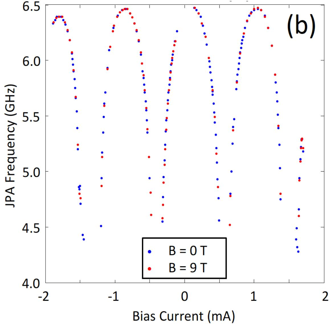
Field at JPA changes  $< 0.01$  flux quantum as the magnet is ramped.
