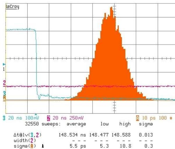
Pulse Width Measurement vs. Simulation
