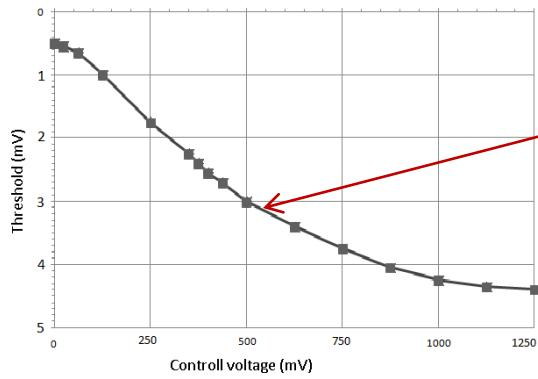
Nonlinear transfer function – especial solution for reduce hard clamping distortion in the amplification stages.
