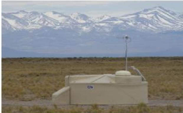
**One of the 1 660 water-Cherenkov detectors (WCD) of the Pierre Auger Observatory, located near Malargüe, Argentina
