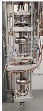
FIG. 1. Left: The experimental setup for the Dark SRF experiment consisting of two 1.3 GHz cavities. Right: A sketch of the Dark SRF electronic system.
